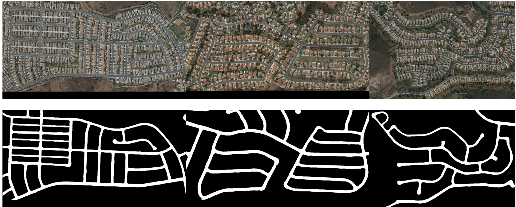
Figure: Examples of the Road dataset along with the corresponding segmentation masks
